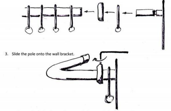
Tighten up the lock collar hex key using the key provided. The screw should go through the hole in the pole and lock into the wall bracket
